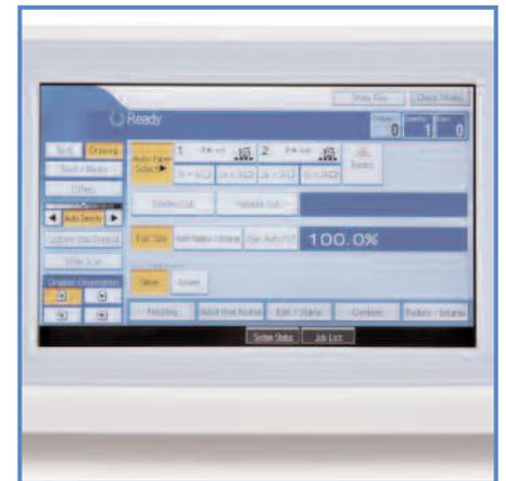
8.5" wide, high-definition LCD control panel—consistent across most Ricoh devices—lessens the learning curve for walk-up users.
